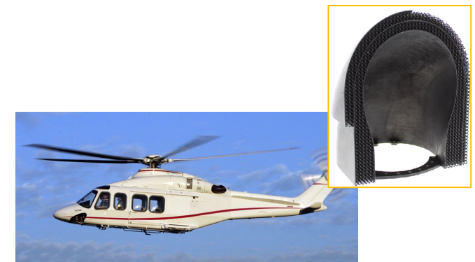
Helicopter exhaust gas nozzle with integral cooling. ( https://altairenligheten.com )
