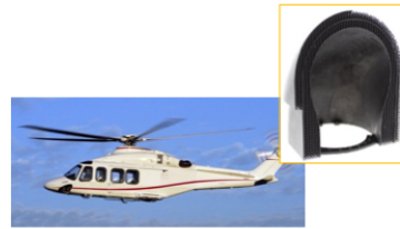
Helicopter exhaust gas nozzle with integral cooling. ( https://altairnlighten.com )
